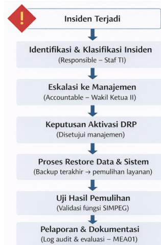
Gambar 7. Alur SOP Pemulihan Sistem ( Disaster Recovery Plan )
