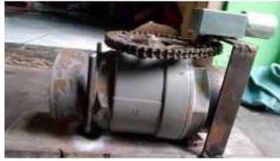
Gambar 3. Motor Operated Valve (MOV) (Anes et al., 2023)
